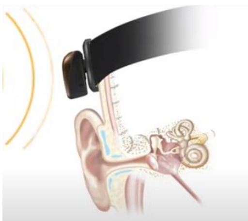
Diagram of bone conduction with a softband. Image courtesy of Cochlear, 2023.
