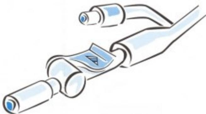
Diagram showing Flip flow valve with Clamp in off position
